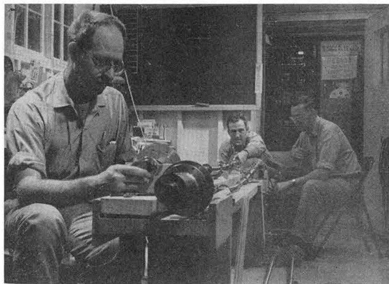
ASSEMBLED long-span displacement gage is calibrated in Sandia shop at Gnome site by R. E. Foster (7251-2), G. W. Burnside (7251-1), and T. B. Morse (7252-1), designer of the gage.
